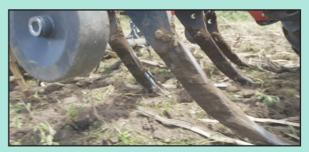
A chisel plough does not turn over the soil. It is better for **Conservation Agriculture**. The seeds will germinate faster and stronger. The soil will not dry out as fast.
