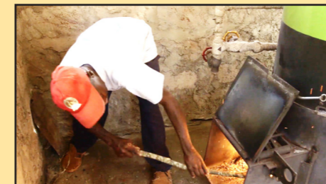
The VIP Drier runs on plant waste like nut shells, saw dust and mango waste.
