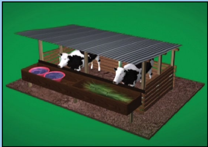
A shed that fits two cows needs to be 12 feet x 10 feet.
