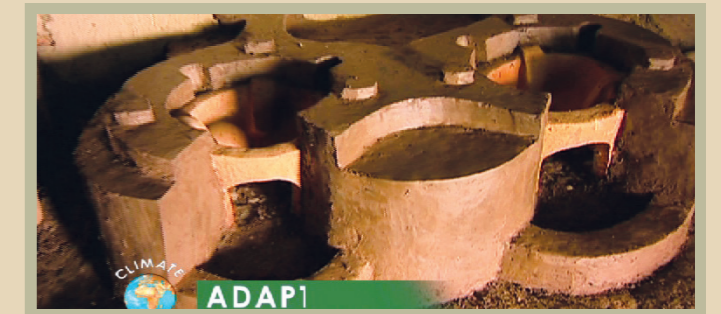
Good jikos use less wood, cook faster, make less smoke and can be put high up.
